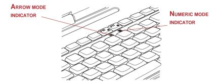
Figure 2-8 Keypad overlay indicators
